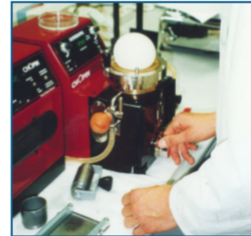
Chopin Alveograph showing stage 5 - air being pumped into dough
